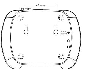
WiFi Reset switch: press and hold down for 10S then release, the blue WiFi indicator will go off and go on again, WiFi setting will be factory reset.
